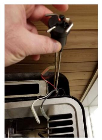
Carefully slide wire connectors off electrodes Pull electrode up and out. Immerse probe in mild decalcifying agent (i.e. CLR) for a period of time.
