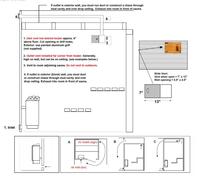
The inlet vent should be driven straight through the wall directly below the center of the heater. The cross-section of the vent for a wall-mounted sauna is approx. 19 sq.in. For larger saunas, approx. 40 sq.in.
