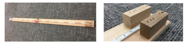
Backside view of a simple valance built from 1x4 cedar with 1x1 stand-off legs.
