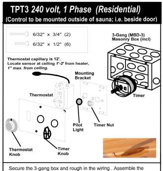
Secure the 3-gang box and rough in the wiring . Assemble the TPT3 Control as shown above; wiring the thermostat, timer and pilot light as per the appropriate wiring diagram.
