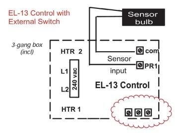
Connect control to external start/stop switch (included) (wire not included).
