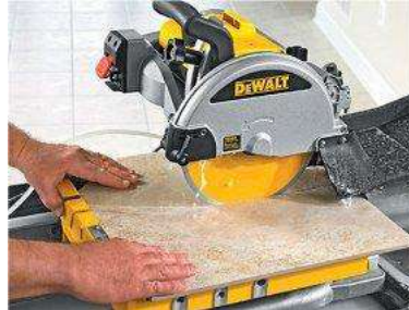
Figure 5.8.1 — A commercial grade wet saw is ideal for cutting all types of tile and stone.
