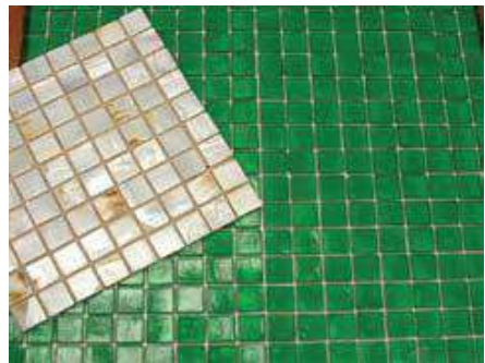
Figure 4.3.1 — Two examples of paperface mounted glass mosaic tile.
