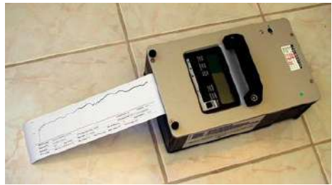
Figure 4.2.1 The BOT-3000 DCOF AcuTest Method apparatus 32
