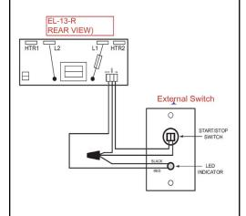
Tylo Pure Control (Not Wi-Fi) with external switch option You must run wire from switch to control.
