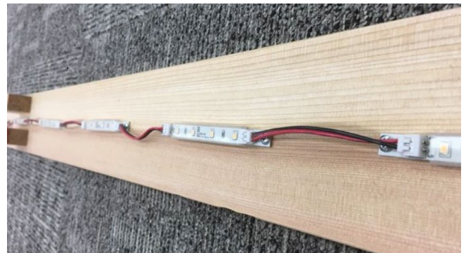
Backside view of a simple valance built from 1x4 cedar with 1x1 stand-off legs.
